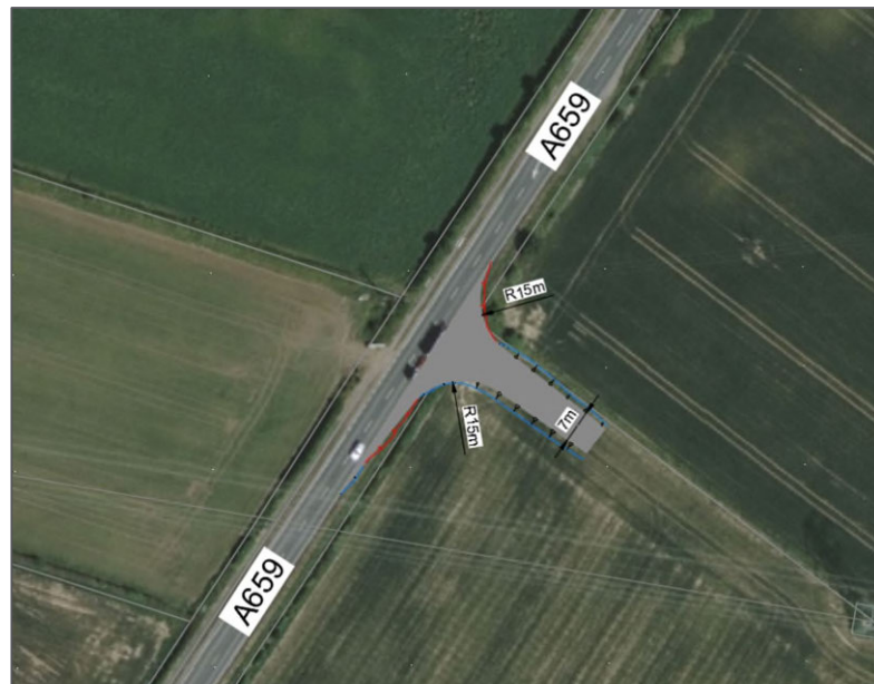
Figure 10: Upgraded Northern Access Bellmouth
