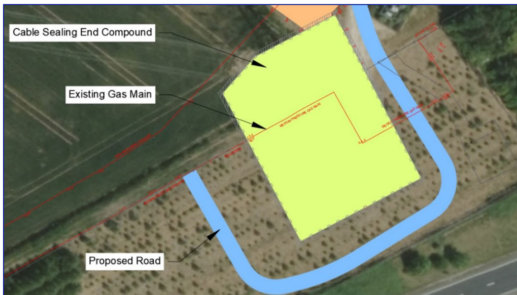
Figure 11: Existing Gas Main Interaction
